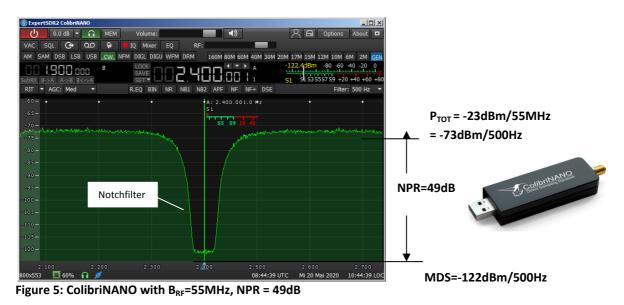
Settings ColibriNANO: Filter 500Hz (CW), MDS -122dBm/500Hz, Attenuation 0dB, Preamplifier off, fs=122.88MHz, Antialiasingfilter fg=55MHz
