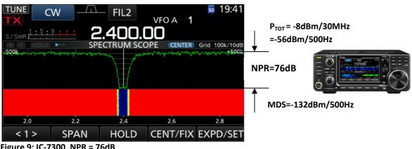
Figure 9: IC-7300, NPR = 76dB
