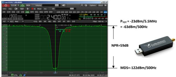
Figure 6: ColibriNANO with B<sub>RF</sub>=5.5MHz, NPR = 59dB
