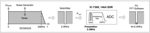
Figure 8: NPR measurement on the IC-7300
