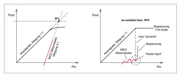
Figure 1: Principle IMD3 curve of an analogue receiver (left) and digital receiver (right)
