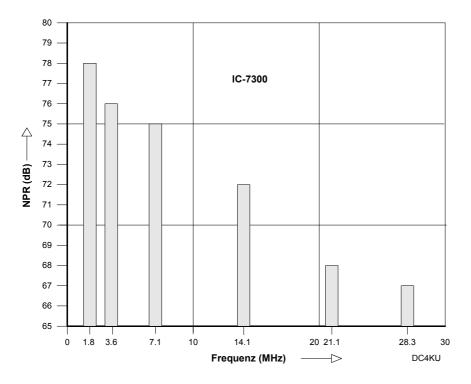
Figure 9: IC-7300, NPR as a function of frequency
