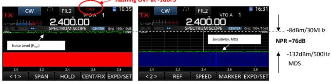
Figure 8: Noise line for clipping (left) and MDS line (right), difference between both lines: NPR
