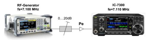
Figure 2 Clipping the IC-7300 by a CW signal
