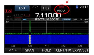
Figure 3: Overflow (OVF) at Pe = -8dBm
