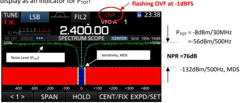
Figure 7: NPR measurement via a notch filter at 2.4MHz
