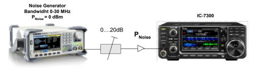
Figure 4: Determining the limitation with a noise signal
