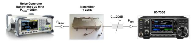
Figure 6: NPR measuring station with notch filter
