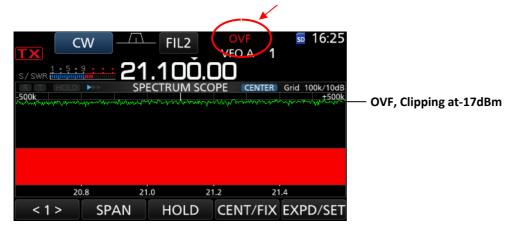
Fig. 5: OVF indication in the 15m band at a noise power line of -17dBm
