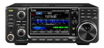
The IC-7300 is a direct-sampling HF/50/70MHz\* transceiver and is characterized by the following features: RF direct sampling, real-time spectrum scope, RMDR 97dB at 1kHz offset, IP+ (dither) function, touch screen color display, built-in antenna tuner and 100 watts transmit power. The features and functions of the IC-7300 have been described in many reports, so that only the most important RF test results will be presented below. \*70 MHz only in Region 1
