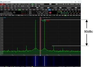
Pi=2x-20dBm, Bandpass-Filter On, IMD3=80dBc ID3 > 20dB above noise (that is too high)
